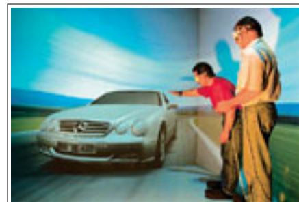
The Cave allows Mercedes designers to work with an almost tangible model. The device is a cube, open at one end, with walls roughly 8.5-feet square. Each wall is a projection screen. The user sits in the center wearing stereovision glasses and data gloves, which transfer movement to the computer.
