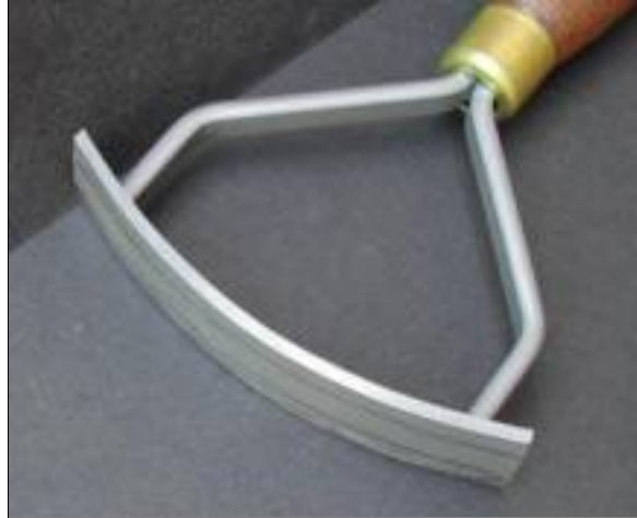
Rake with horizontal lines draw on the blade to guide grinding the blade into a steeper angle.
