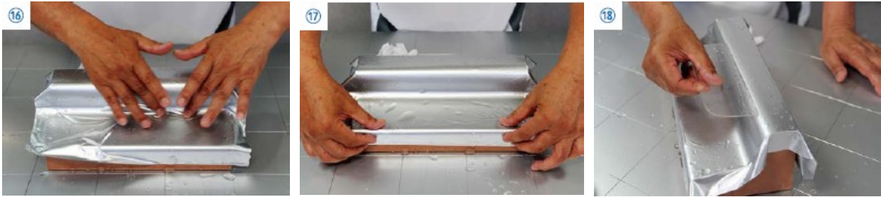
Adjust the film's position, removing the water and foam from under the film with a rubber spatula or squeegee. Then it will adhere to the surface of the clay surface.
