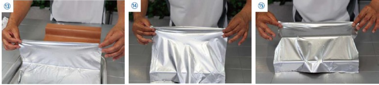
First moisten the surface of the clay by spraying it with water. Then carefully cover the clay model with the film.
